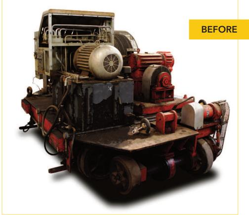
The powered trolley required stripping, repairing and an upgrade of the electrics and hydraulics systems in order to extend the lifetime and improve the reliability of this safety-critical asset.
