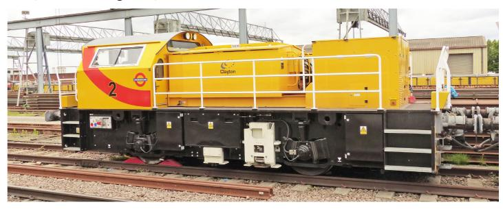
Conversion of ten Diesel locomotives to zero emission battery locomotives, complete with on-board charging. Also, to operate from both the on-board traction battery and the 3rd/4th rail supply.
