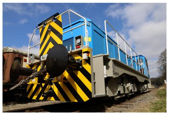
As part of Tata Steel's requirement to replace their ageing locomotive fleet at the Port Talbot works, Tata Steel has ordered a number of new battery hybrid locomotives, designed and manufactured by Clayton Equipment.
